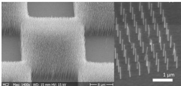
Left: nanostructures grown in “checker box” pattern
