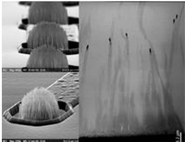
Left: nanostructure bumps grown from Al metal pads
