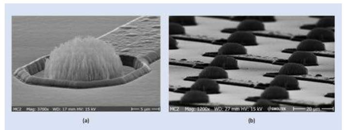
Figure 5: (1.) An SEM micrograph of carbon bumps grown (hence rooted) on solder pads and (2.) an array of carbon bumps.
